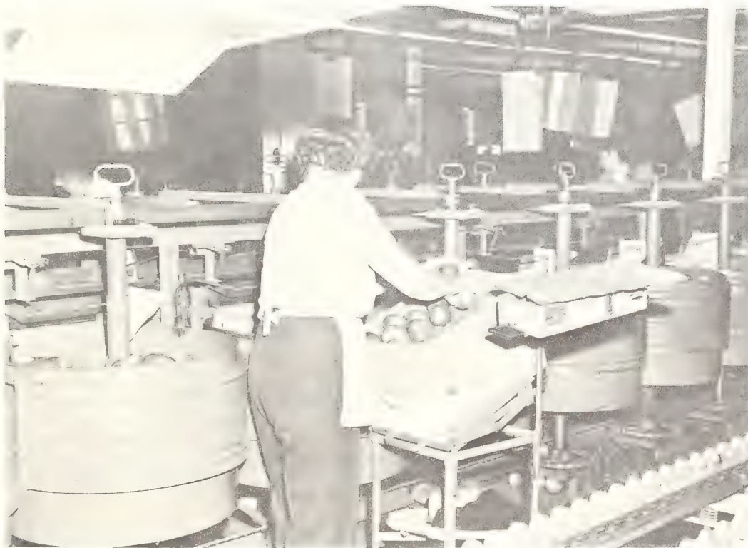
Figure 19.--Packing trays by hand from a rotating tub. A "floating" bottom holds apples at a fixed height for ease of packing.
