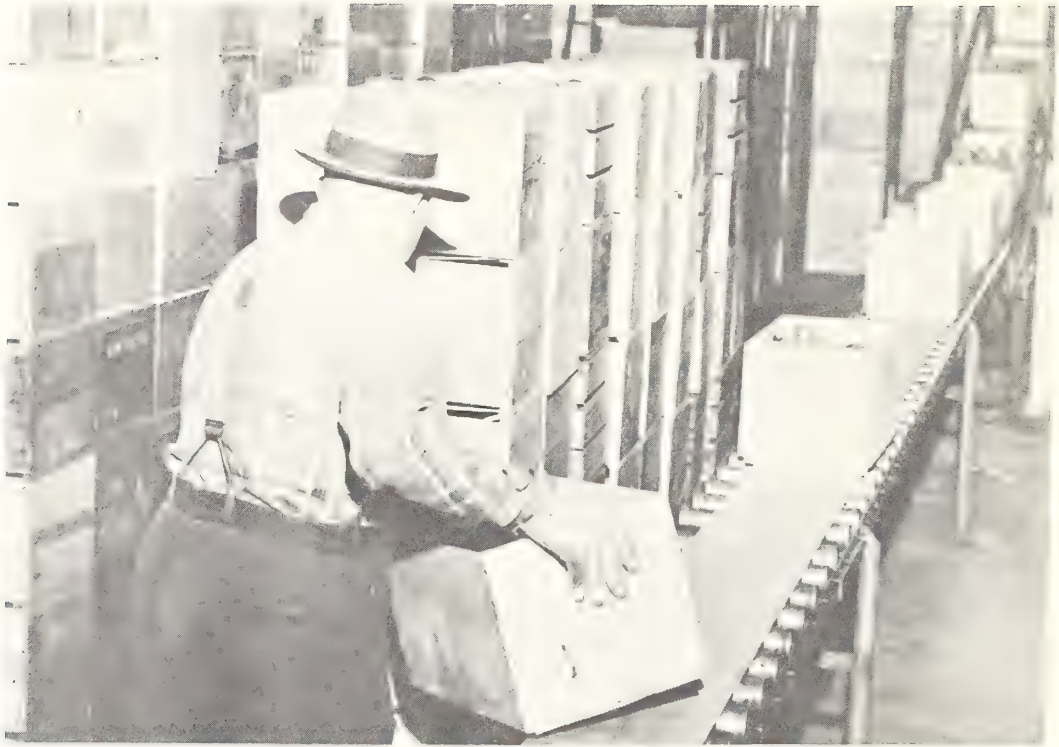
Figure 4.--Five-high stacks alongside conveyor. These stacks are built manually with crates taken from the conveyor. They are later removed by clamp type 2-wheel handtruck.
