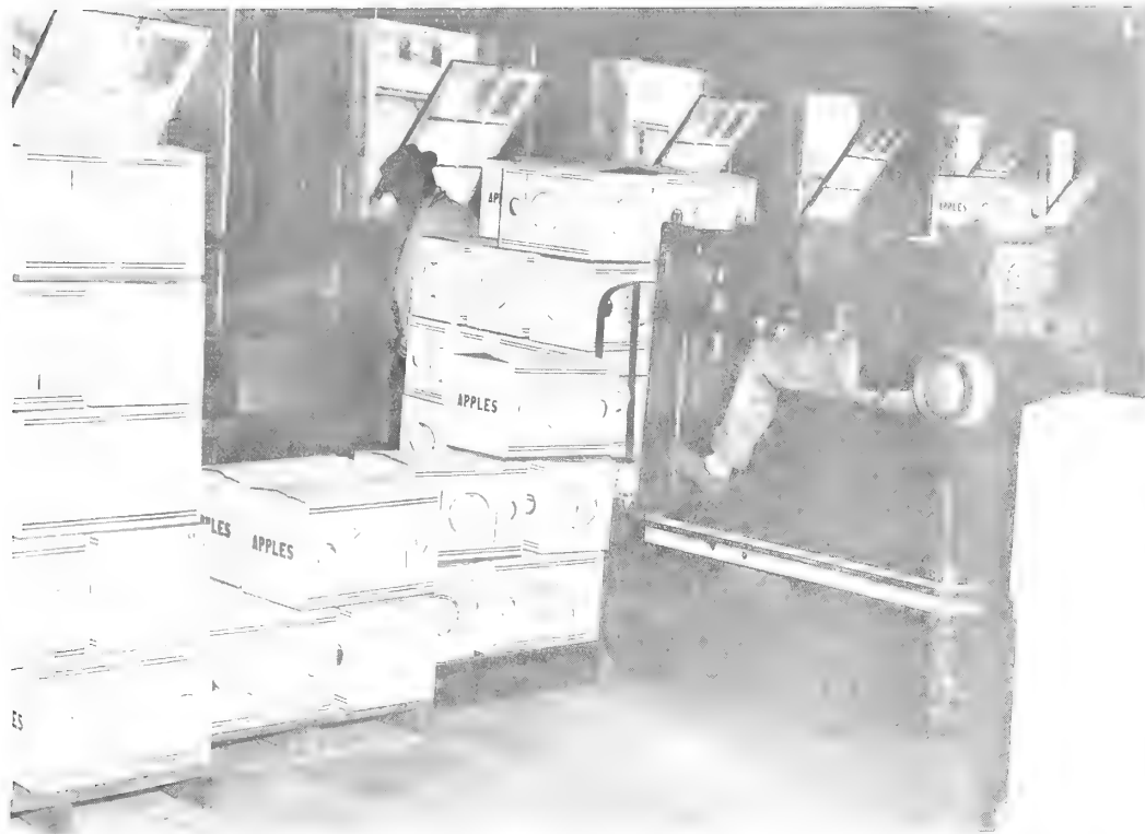
Figure 9.--Segregating onto pallets. One worker removes cartons from conveyor and places them on designated pallets. Forklift truck removes full pallets.
