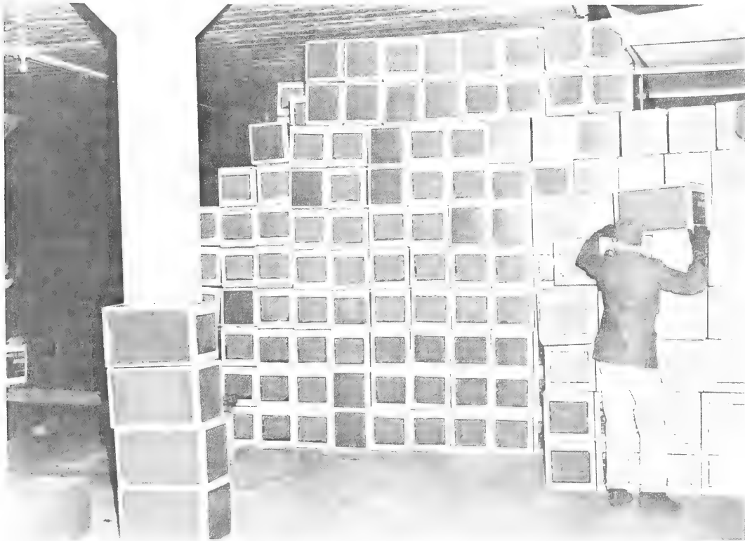
Figure 10.--A manual stacking operation. Worker removes carton from conveyor, carries it to the stack, and places carton in storage.
