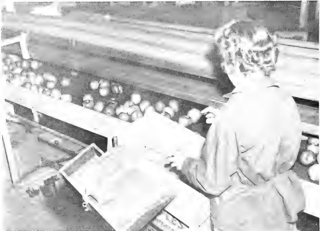
Figure 20.--Worker manually packing apples from a return-flow belt.
