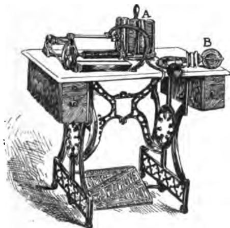
FIG. 3.—THE PHONOGRAPH-GRAPHOPHONE. A, cylinders; B, recording diaphragm with speaking-tube attached.
