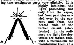
but from particles carried over by the current and from the heated ends of the broken circuit (electrodes). In the ordinary arc light the electrodes are carbon rods, with a mechanism for maintaining them at a small, constant distance. When the carbons are saturated with
