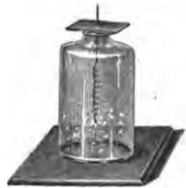
COMBUSTION OF IRON IN OXYGEN.
