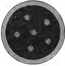
UNDERGROUND CABLE, CONTAINING SIX-STRANDED CONDUCTORS FOR ELECTRIC LIGHTING.
