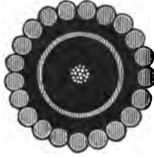
SUBMARINE CABLE, WITH ONE-STRANDED CONDUCTOR.
