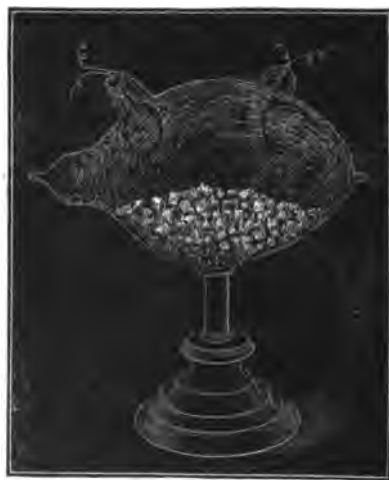
A CROOKES TUBE, SHOWING LUMINESCENCE OF CRYSTALS, UNDER ACTION OF KATHODE RAYS.
