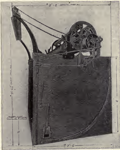
FIG. 117.—Roll Machine for Bleaching Knitgoods.
