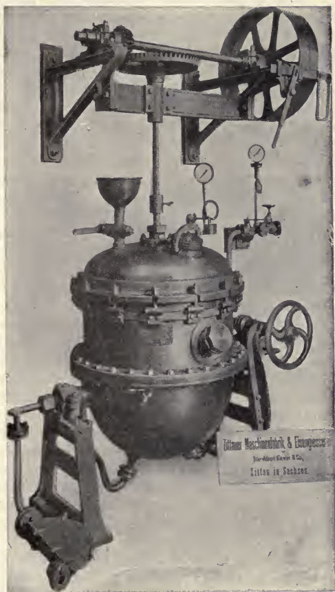
FIG. 122.—Autoclave (Pressure Kettle) for Preparing Dyewood Solutions.
