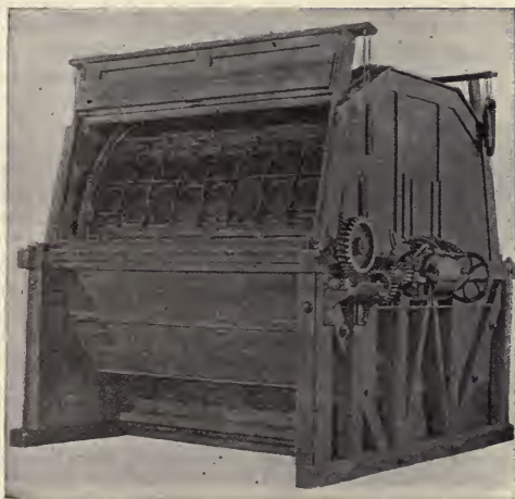
FIG. 119.—Raw Stock Bleaching Machine. (Delahunty Dyeing Machine Co.)
