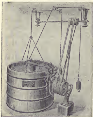
FIG. 126.—Dyeing Machine for Loose Stock. (Esser.)
