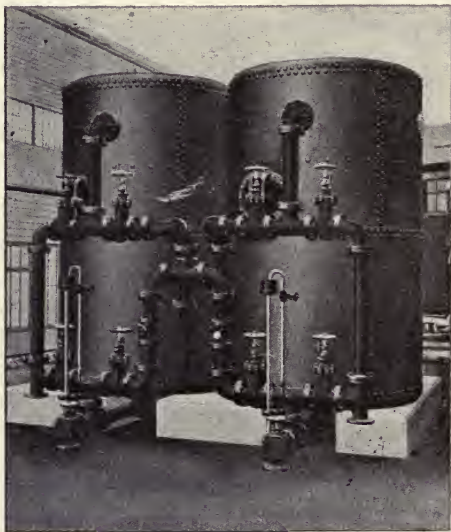
FIG. 92.—Water Softener. (Permutit System).
