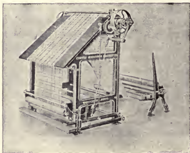
FIG. 289.—Cloth-inspecting Machine with Cradle, Reverse Motion, and Rolling Head. (Curtis & Marble.)
