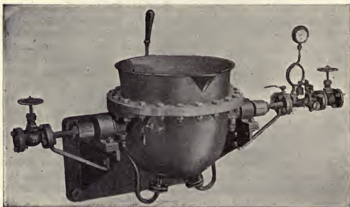
FIG. 121.—Modern Type of Kettle for Preparing Solutions for Dyeing.
