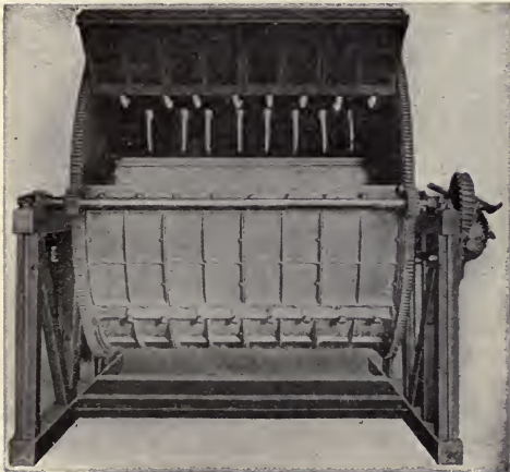
FIG. 22.—Revolving Cylinder Type Raw Stock Dyeing and Bleaching Machine. (Delahunty Dyeing Machine Co.)
