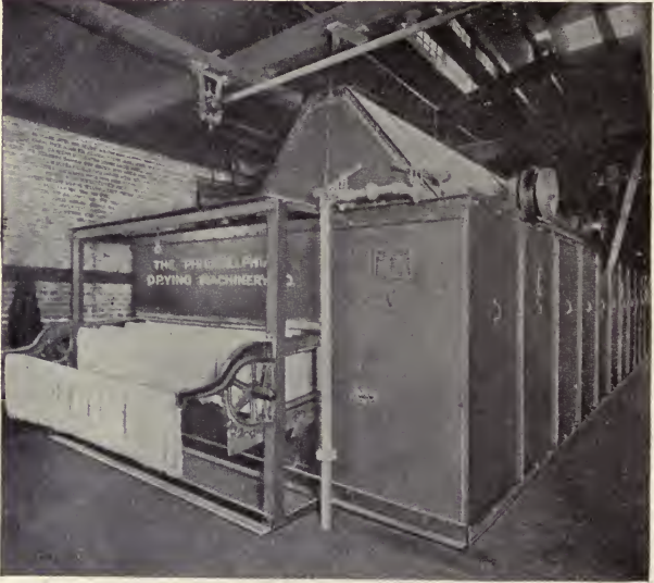
Fig. 49.—Automatic Yarn Dryer with Thermostatic Temperature Control. (Philadelphia Drying Machinery Co.)
