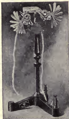
FIG. 282. — Quartz Ultra-Violet Lamp for Testing Fastness of Colors to Light. (Hanovia.)
