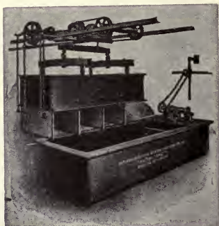
FIG. 165.—Circulating Dyeing Machine for Hosiery. (Philadelphia Dyeing Machine Co.)
