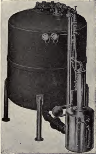
FIG. 83.—Pressure Kier with Vacuum Circulation. (Jefferson Patent.)
