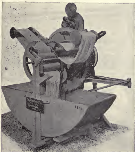
FIG. 230.—Impregnating Machine for Yarn. (Haubold.)
