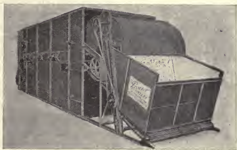
FIG. 133.—Automatic Dryer for Cotton, Wool, Raw Stock, etc. (Philadelphia Textile Machinery Co.)
