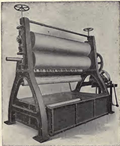
FIG. 101.—Bleach House Washer. (Textile-Finishing Machinery Co.)
