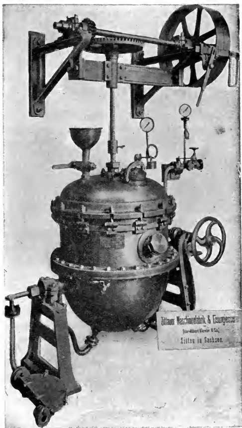
FIG. 122.—Autoclave (Pressure Kettle) for Preparing Dyewood Solutions.
