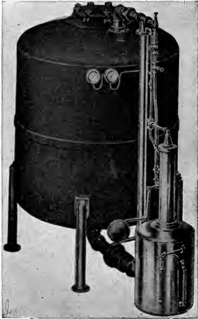
FIG. 83.—Pressure Kier with Vacuum Circulation. (Jefferson Patent.)
