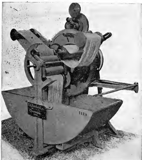
FIG. 230.—Impregnating Machine for Yarn. (Haubold.)
