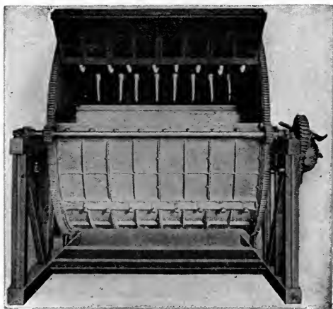
FIG. 22.—Revolving Cylinder Type Raw Stock Dyeing and Bleaching Machine. (Delahunty Dyeing Machine Co.)
