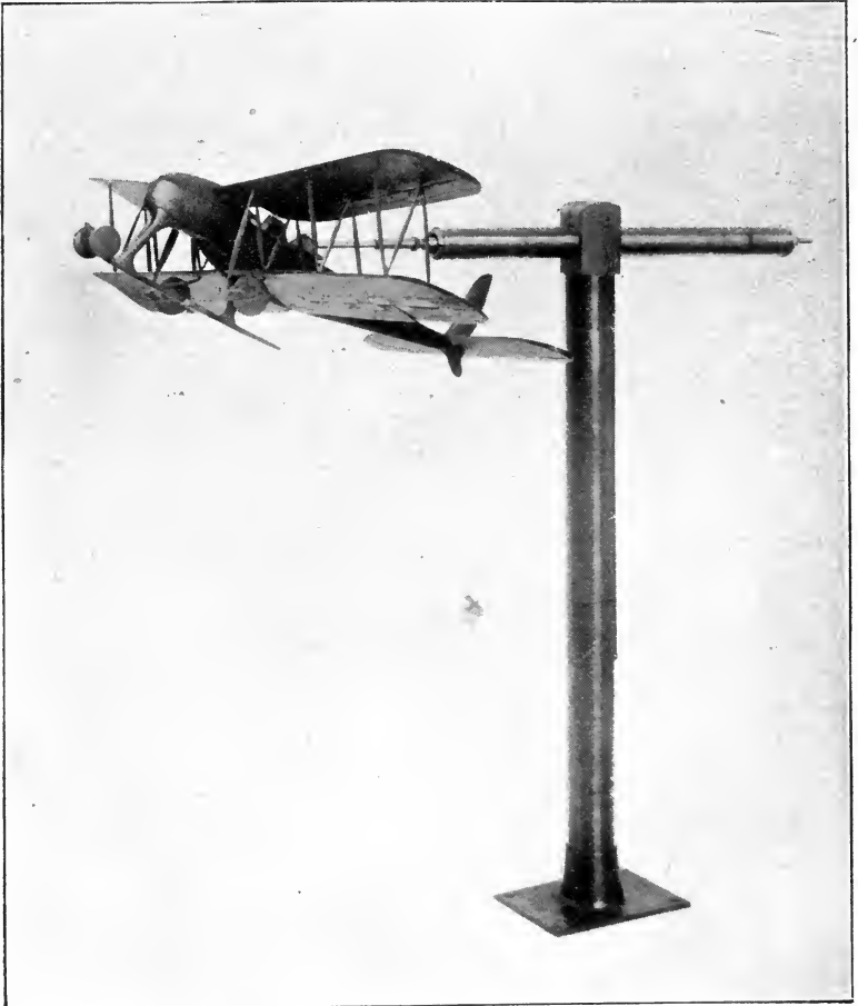
FIG. 136.—Model aeroplane arranged to show autorotation.
