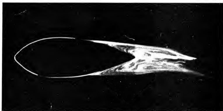
FIG. 174.—Eddying motion behind medium strut (N.P.L.).
