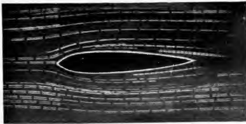
FIG. 172.—Viscous flow round strut section (free fluid).
