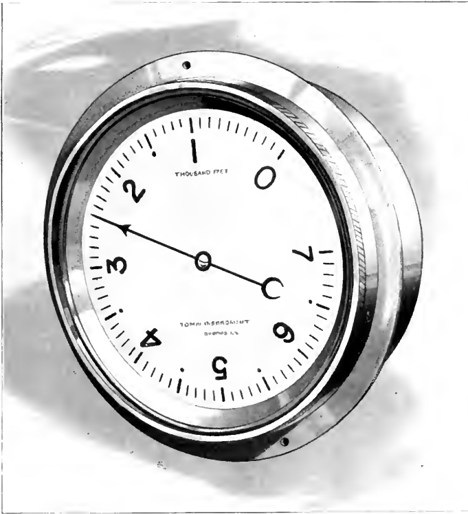
Fig. 55—Altimeter as used on airplanes
