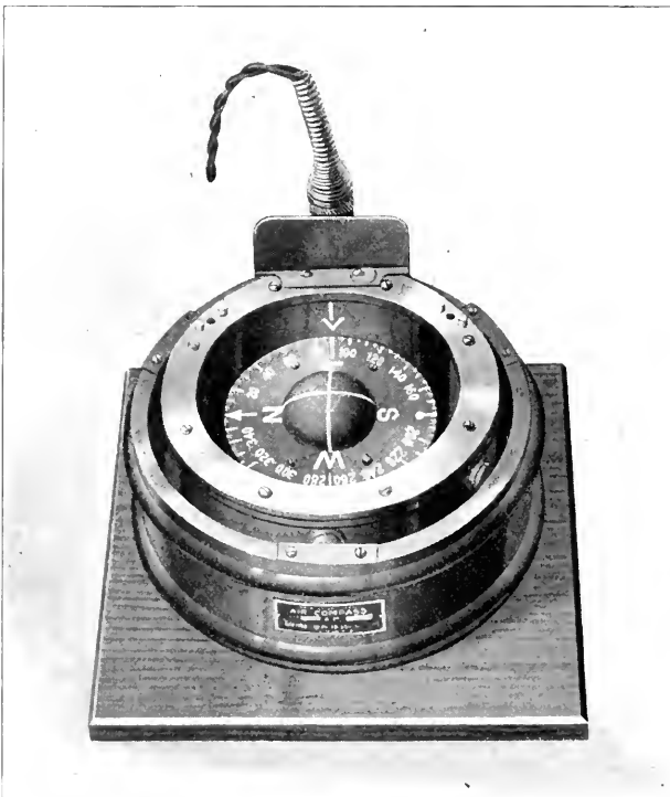
Fig. 53—Creagh Osborne type of airplane compass
