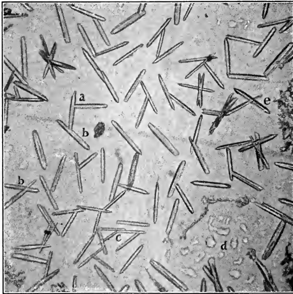
FIG. 421. Cubebin: orthorhombic crystals from Prollius' solution, showing various types of twinning (a, b, c); d, amorphous material in the form of oily drops (under-cooled liquid); e, this amorphous material crystallizing in aggregates.
