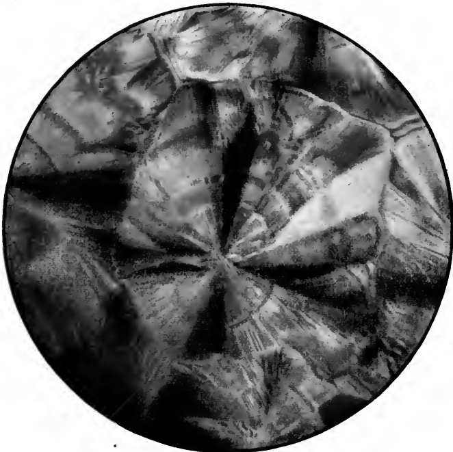
FIG. 100. Cocaine hydrochloride. Aggregates from aqueous solution. CRYSTALS IN POLARIZED LIGHT (Crossed nicols).
