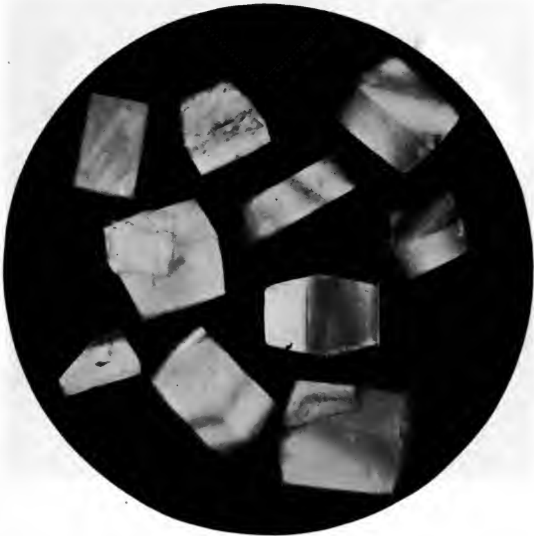
FIG. 422. Strychnine sulphate: tetragonal crystals in polarized light, showing side aspect.
