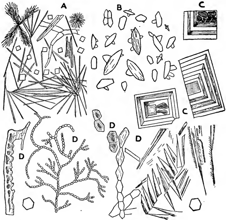
FIG. 419. Crystals of some of the common reagents which not infrequently separate on the slide and may be mistaken for cell contents: A, isotropic crystals of chloral which occur in cubes about 10\ \mu in diameter or long needles about 50\ \mu long; B, phloroglucin which occurs in broad rectangular plates or ellipsoidal discs from 10 to 35\ \mu in diameter which are doubly refracting with a play of colors; C, cubes of potassium iodide which are isotropic; D, crystals from potassium hydrate solution which separate in broad prisms and branching chains that are doubly refracting and give marked color effects.
