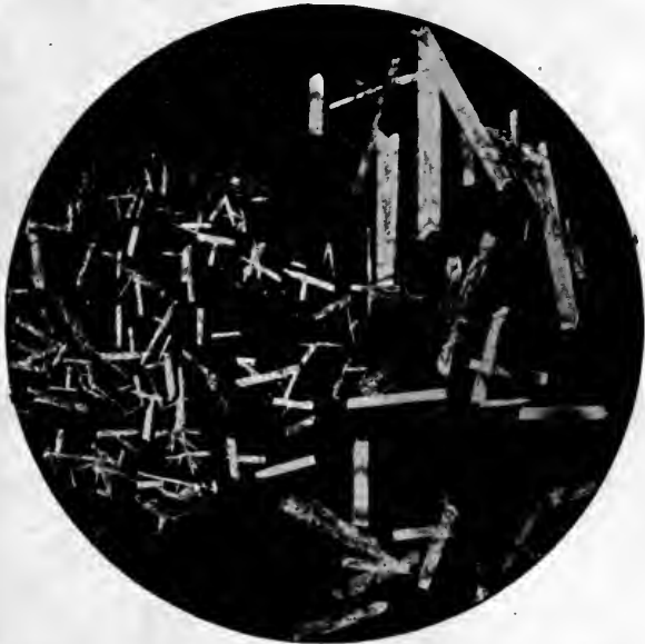
FIG. 96. Caffeine gold chloride; crystals formed on the addition of a solution of gold chloride to a dilute aqueous solution of caffeine.
