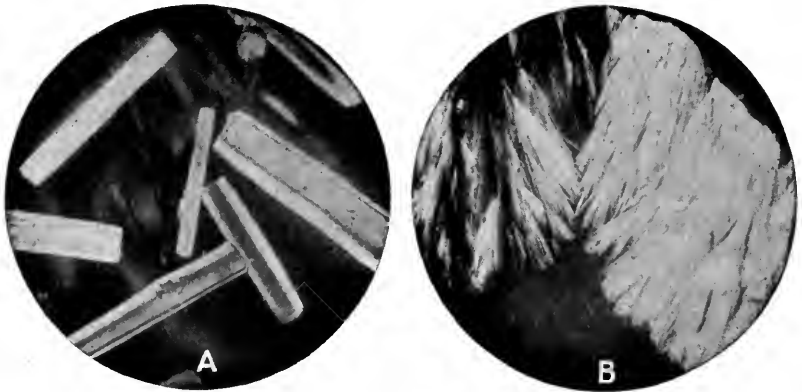
FIG. 94. Orthorhombic crystals of Mannitol (Mannit) obtained from aqueous solutions: A, large crystals; B, feathery aggregates of needles.
