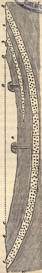
FIG. 12.—Illustration of Artesian Wells. (After Chamberlin.)
