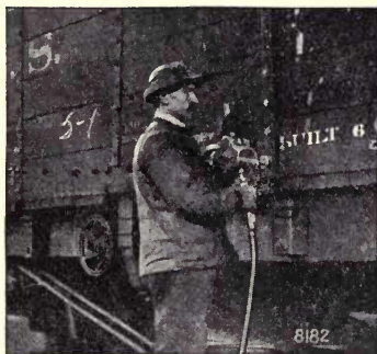
FIG. 8.—A power tool (compressed air attachment) tightening nuts on a freight car. Compressed air may be utilized in this way to screw on nuts and thus save the mechanic's strength.
