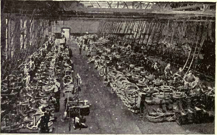
FIG. 109.—A Nail Factory. The wire is fed into machines which cut and shape the wire into nails.
