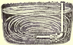
FIG. 157. —Heating Water by Steam. The arrow represents the passage of heat (by steam) into the water. The attachment is screwed onto the steam pipe.
