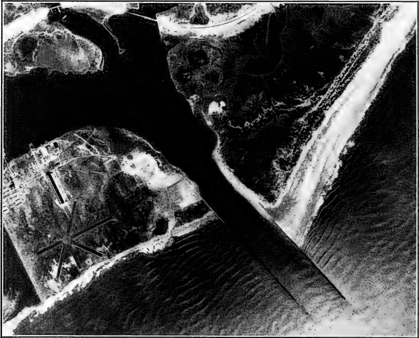
FIG. 2. Cold Spring Harbor, New Jersey. A wide beach has been formed by material trapped by jetties (right). The downdrift beach (left) is starved and subject to serious erosion. April 1940. (Photo by Aero Service Corp.)
