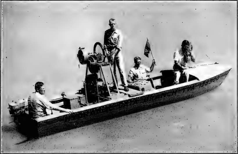
FIG. 3. Sounding boat on reservoir survey. The man in the bow maintains shore contact with a hand radio, the man with the flag operates the echo-sounding recorder, the man standing operates a device that measures distance from shore by a taut piano wire, and the man in the stern operates the outboard motor that powers the boat.
