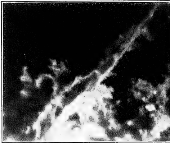
FIG. 7. Plastic model of fractured carbonate rock (Devonian), showing secondary ground-water solution. South Fullerton Field, Andrews County, Texas. Magnification 10 \times . (From Imbt and Ellison, 1946, p. 366.)
