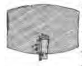
Section showing the method of fastening the method of fastening. Weight of stone 5600
