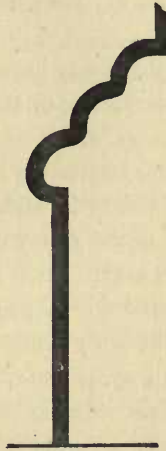
Ripon Cathedral Church, bases of vaulting shafts of choir aisles, Geometrical, 1288-97.
