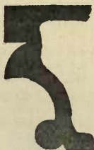
Ripon Cathedral Church, abacus moulds of capitals, north and south arcades of choir (reproduced in 15th cent).
