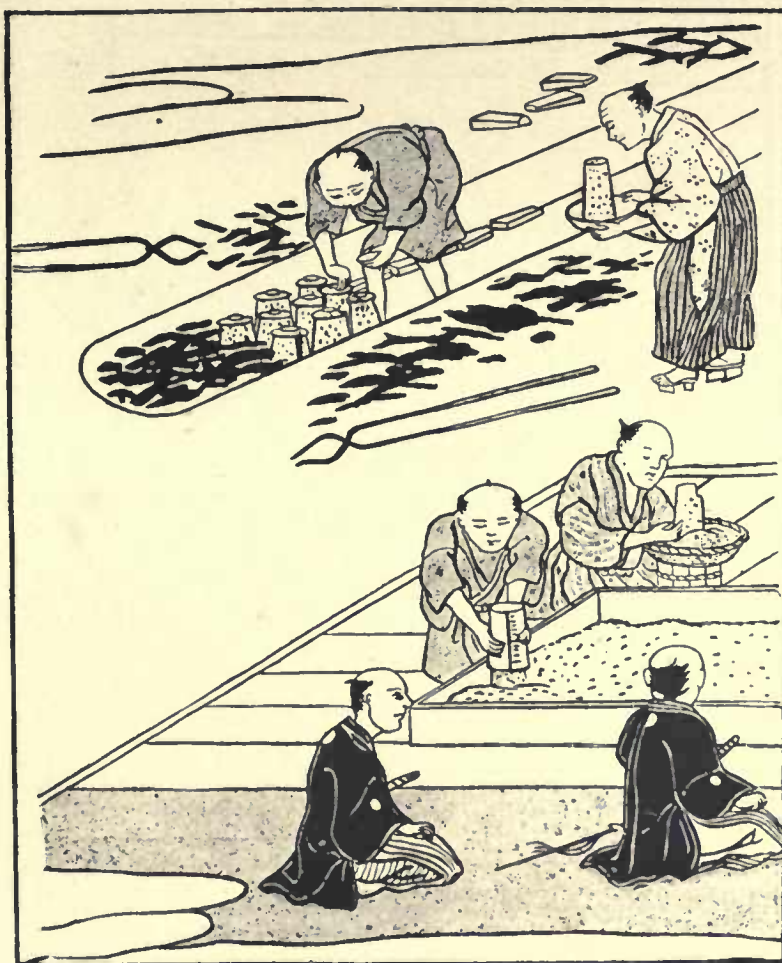
Fig. 3. Charging the furnace. Japan.
