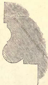
Section of Side Arch at C. D.
