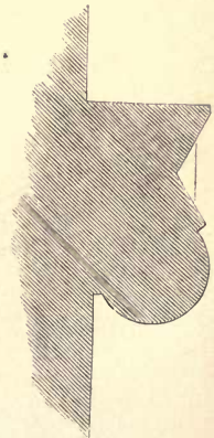
Section of Impost Mouldings.
