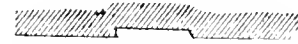
Details of the groove cut on each side of the course A. HORIZONTAL SECTION. Scale \frac{1}{10} .
