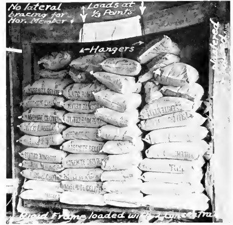
TEST OF FABRICRETE RIGID FRAME
