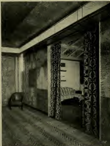
MEN'S SMOKING ROOM—Walls and ceiling, Hungarian ash crotch veneer with Prima-vera trim. Floor tile in russet brown tones. Drapes, tan and silver. Illuminated frieze is opal glass
