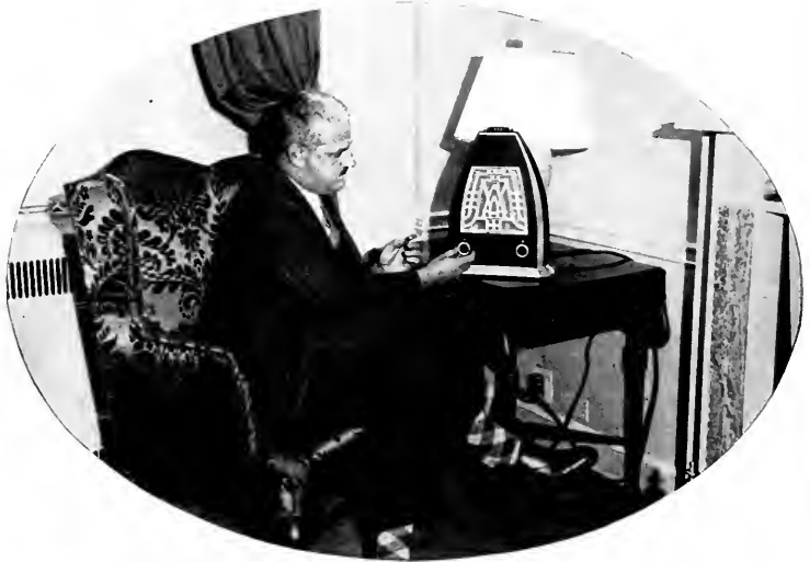
Room guest selects one of the six programs made available through the hotel's radio distribution system and this specially designed loudspeaker
