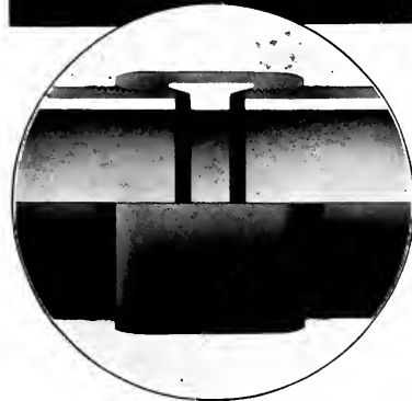
Section of National DUROLINE Pipe coupling and joint. (Note special high-strength corrosion-resistant joint compound on end of pipe and on threads).
