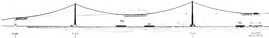
FERRIED ON BARGES roadway trusses for the Bay Bridge are lifted from barges, into position and fastened to suspender cables as shown in sketch.
