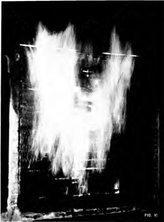
FIG. 10 FIRE TESTS OF VERTICAL PANELS OF RED OAK—NOT TREATED EXPOSED FACE WHEN WITHDRAWN FROM FURNACE
