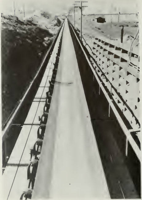
EIGHT LAYERS OF COTTON FABRIC USED IN THE MANUFACTURE OF THIS 9,700 FT. GOODYEAR BELT
