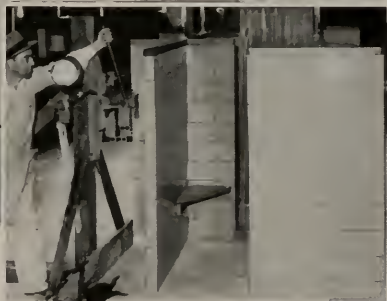
Vallejo, California. High School. John J. Donovan, architect. Reed & Reed, masonry contractors. Inset photograph shows preliminary testing of Kraftile Terra Cotta Wall Unit reinforced partitions in Kraftile plant at Niles, California
