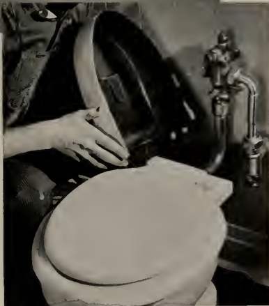
The streamlined housing which covers the flush valve is easily removed for inspection. The entire combination is compact and space-saving, roughing-in normally at 10" with ample tolerances for both water and waste connections.
