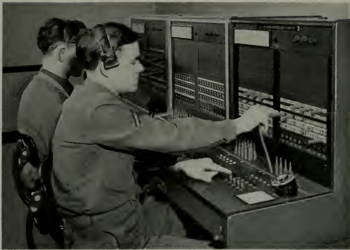
AIR RAID WARNING SWITCHBOARD —Here the C. A. R. W. officer at each Army Information Center notifies designated civilian district warning centers of the approach of enemy planes. Note that there is a group of four jacks for each warning center: three to report differing degrees of danger, and the fourth to transmit the "all clear"
