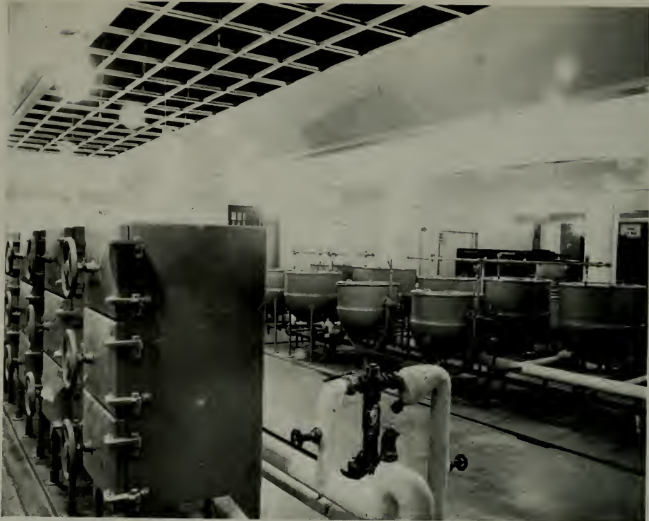
TWO ROWS OF GIANT KETTLES OPERATE LIKE DOUBLE BOILERS, UTILIZING STEAM RATHER THAN BOILING WATER FOR LIQUID COOKING
