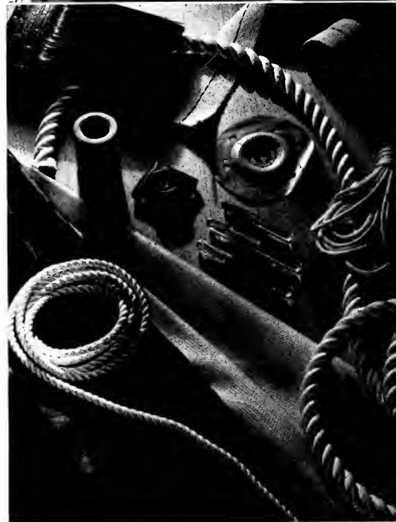
Upper right: Plastic nose for a Martin bomber. Lower: Nylon plastic for post-war industry—rope, parachute cloth and bristles.
