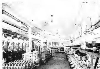
Sound conditioned assembly and motor test room, Caterpillar Tractor Co., San Leandro
