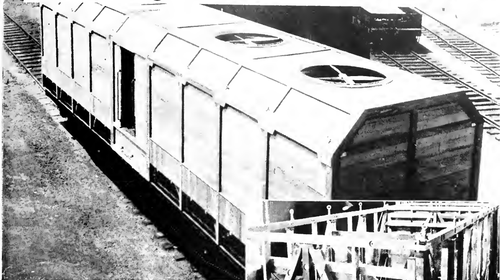
↑ Completed Foster Wheeler built cooling tower car ready for coupling to rest of power train.
