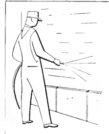
1. Structural wall is wet; Ceramic Veneer soaked.
