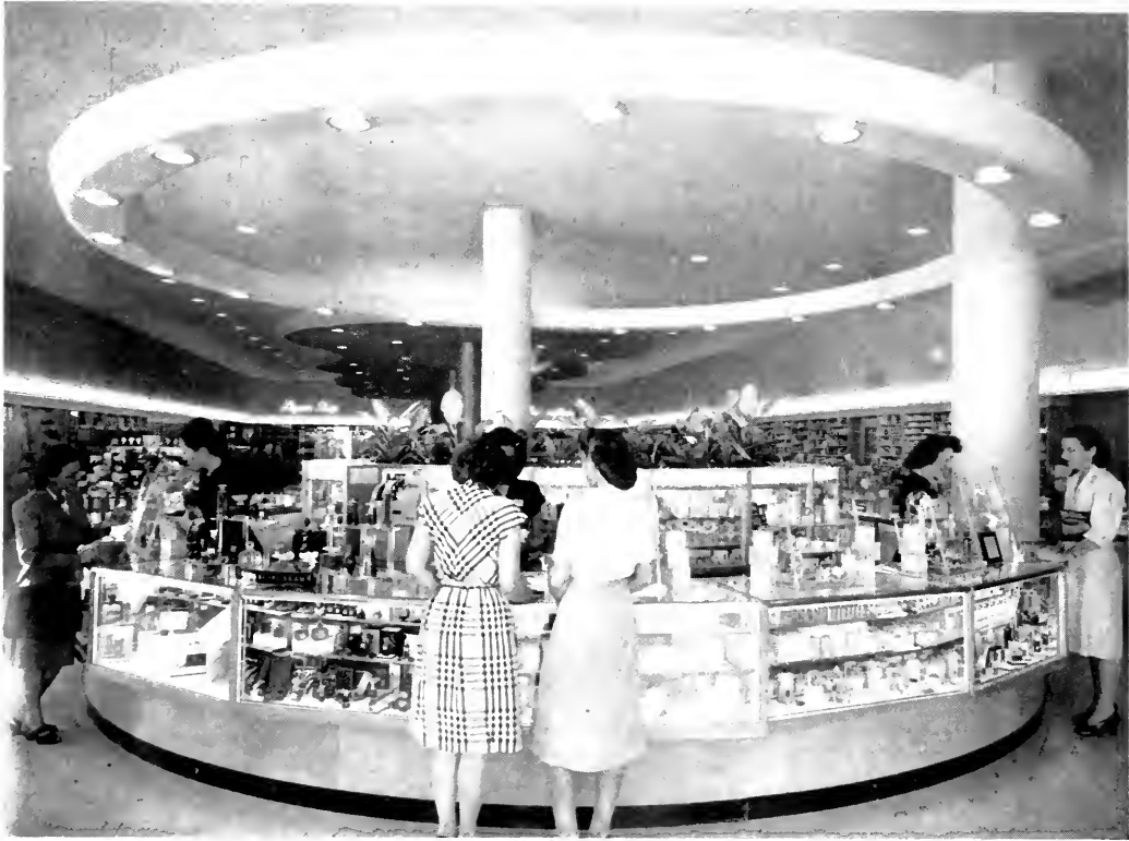
ABOVE: Beauty Bowl in the new Owl Rexall Super Drug Store. Circular light trough overhead has one soft spotlight for each of the 17 sectional cases.
