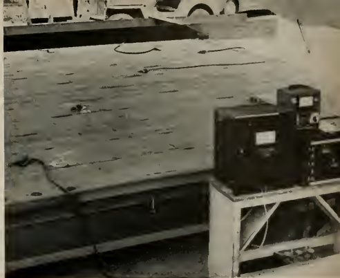
Electric strain gauges were used to check stress imposed on Fenestra Building Panels by the lateral load.
