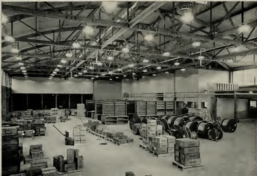
Interior of warehouse with post-free work area of 100x180 feet. A bay of windows around the entire warehouse section provides daylight.
