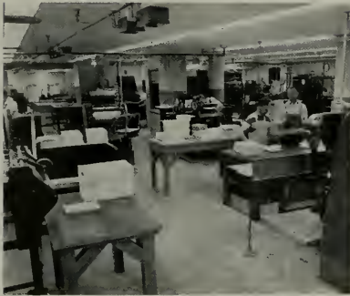
Production Department: Showing some details of building installations—wooden block floor, ventilation ducts in ceiling, and recessed fixtures for all lights.
