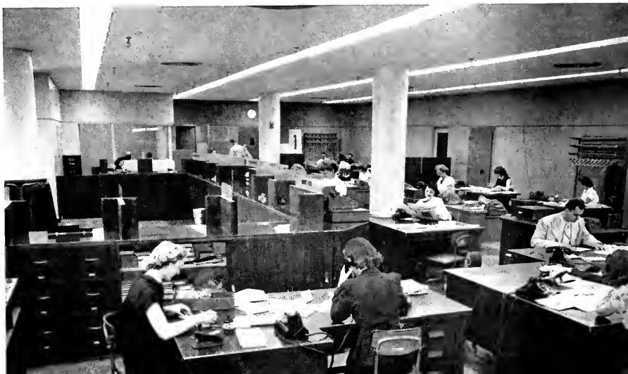
BUSINESS OFFICE: Showing Public counter at left center. Acoustical tile ceiling reduces noise and recessed lighting eliminates eye strain.
