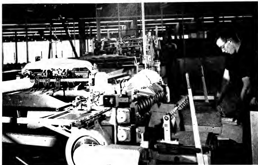
MAKING LITTLE ONES OUT OF BIG ONES —Modern slitter machine cuts large sheets of tinplate into "body-blanks" of exact size of the tin cans to be made.
