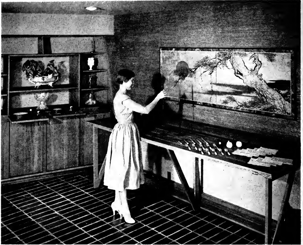
A wainscoting wall section in the home of Mr. and Mrs. Sam Rubenstein tips up to form this remarkable buffet table, a real space saver in a busy family room. Thomas A. Balshizer, Architect.
