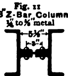
Fig. 12 6" Z-Bar Column \frac{1}{2} to \frac{3}{4} " metal
