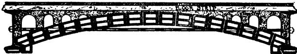
4' to 6' Segmental Arch. Weight of tile 24 to 36 Lbs. Span to 16 to 20' according to size of beam.
