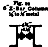
Fig. 11 8" Z-Bar Column \frac{1}{2} to \frac{3}{4} " metal
