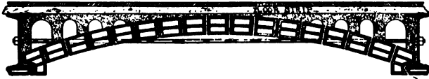
4' to 6' Segmental Arch Weight of tile 24 to 36 Lbs. Span 6' to 200' according to size of head
