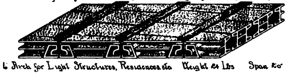
Transverse System of Floor Arch Construction Weight of tile 25 to 40 Lbs. Span 6' to 120'
