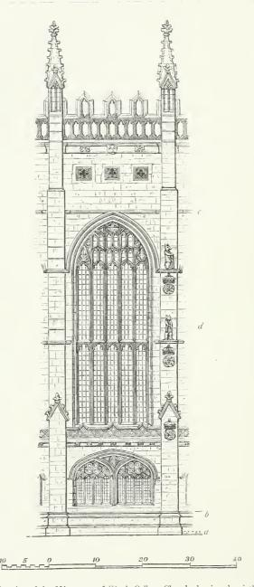
Fig. 43. Elevation of the fifth severy of King's College Chapel, shewing the sixth and seventh buttresses on the north side (fig. 42).
