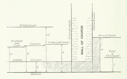
Fig. 14. Diagram to show the "enhancing" of the site of Eton College. Scale  $\frac{1}{4}$ th of an inch to one foot.
