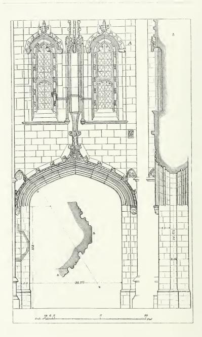
Fig. 10. Elevation of the interior of the Gateway, Old Court of King's College, after Pugin.
