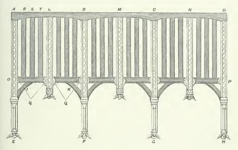
Fig. 13. Elevation of the roof, according to the contract, 1452.
