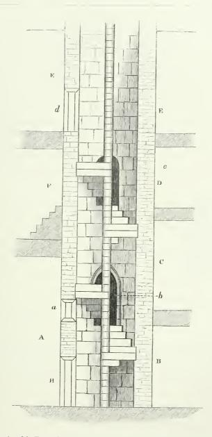
Fig. 6. Section of the Turret, drawn along the line OP, fig. 2. A. Hall. B. Combination Room. C. Andit Room. D. Room above the last, occupied as a College Room. EE. Garrets. F. Library. H. Door leading into the Hall. a. Window looking into the Hall. b. Door leading to the Audit Room. c. Door leading to the Rooms above the Audit Room. d. Door leading to the Garrets above the Library.
