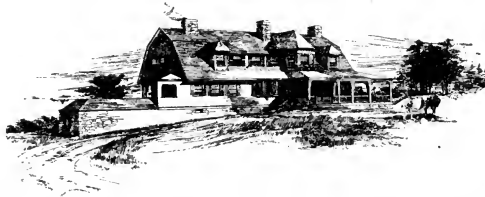
265. House at Little Harbor, N. H. The dormers are arranged as an unsymmetrical triple group.
