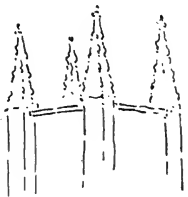
23. Four-pinnacled tower, a type to be avoided.
