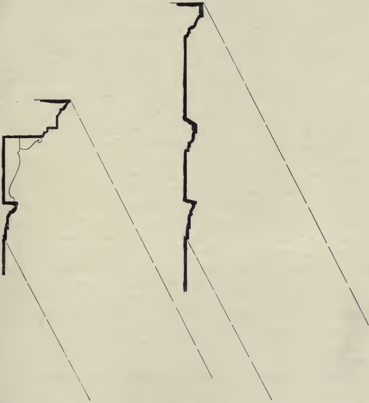
Fig. 2.—A Vertical Cornice-Member, 14 Feet High, Subtending the Same Angle as a Wall Cornice, 9 Feet High and of 4 Feet Projection.
