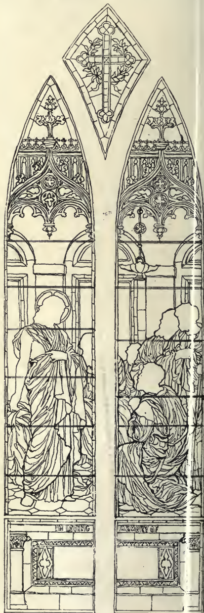
"LEADING" PLAN FOR WINDOW IN CHURCH OF THE ASCENSION, N. Y.
