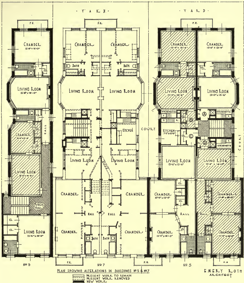
FIG. 23. PLANS SHOWING ALTERATIONS OF "OLD TYPE" NARROW APARTMENTS INTO MODERN SMALL APARTMENTS. 5, 7 AND 9 WEST SIXTY-FIFTH STREET, NEW YORK. Emery Roth, Architect
