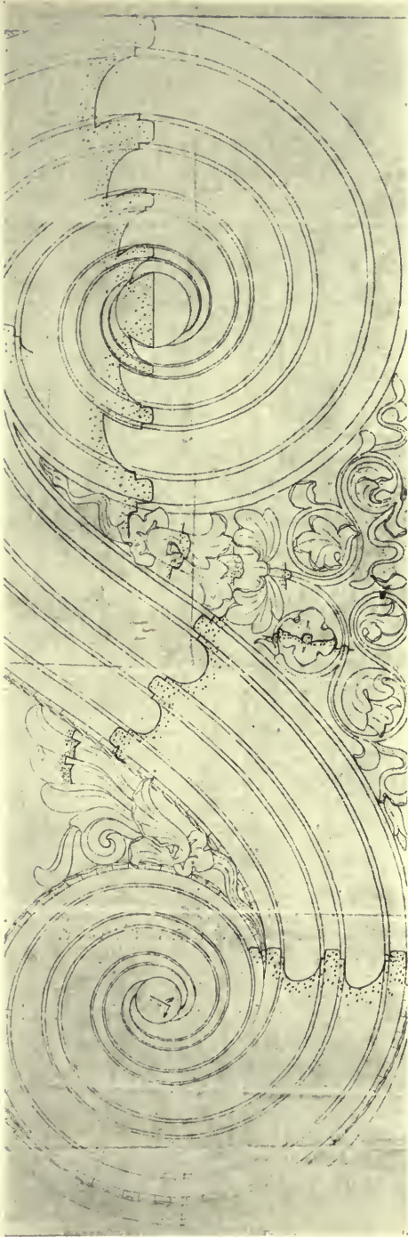
DETAIL, SIDE ELEVATION OF CONSOLE FOR MAIN ENTRANCE — SEABOARD NATIONAL BANK, NEW YORK. Alfred C. Bossom, Architect.
