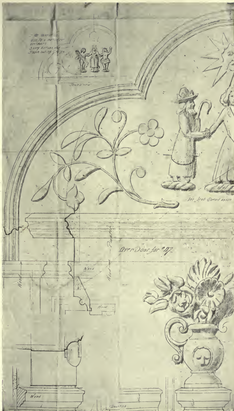
DETAIL OF PLASTER WORK IN HALL—RESIDENCE OF THOMAS W. LAMONT, ESQ., NEW YORK CITY. WALKER & GILLETTE, ARCHITECTS.
