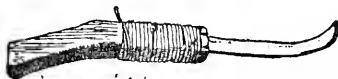
Bess-hath or crooked knife. 10\frac{1}{2} in. long. Property of Weeso. Made of a file. July 16, 1907
