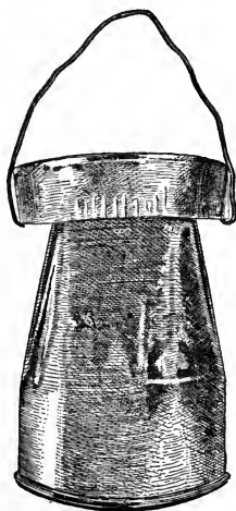
FIG. 5.—Tin can container for ant-poison sirups used in outdoor experiments. (Original.)
