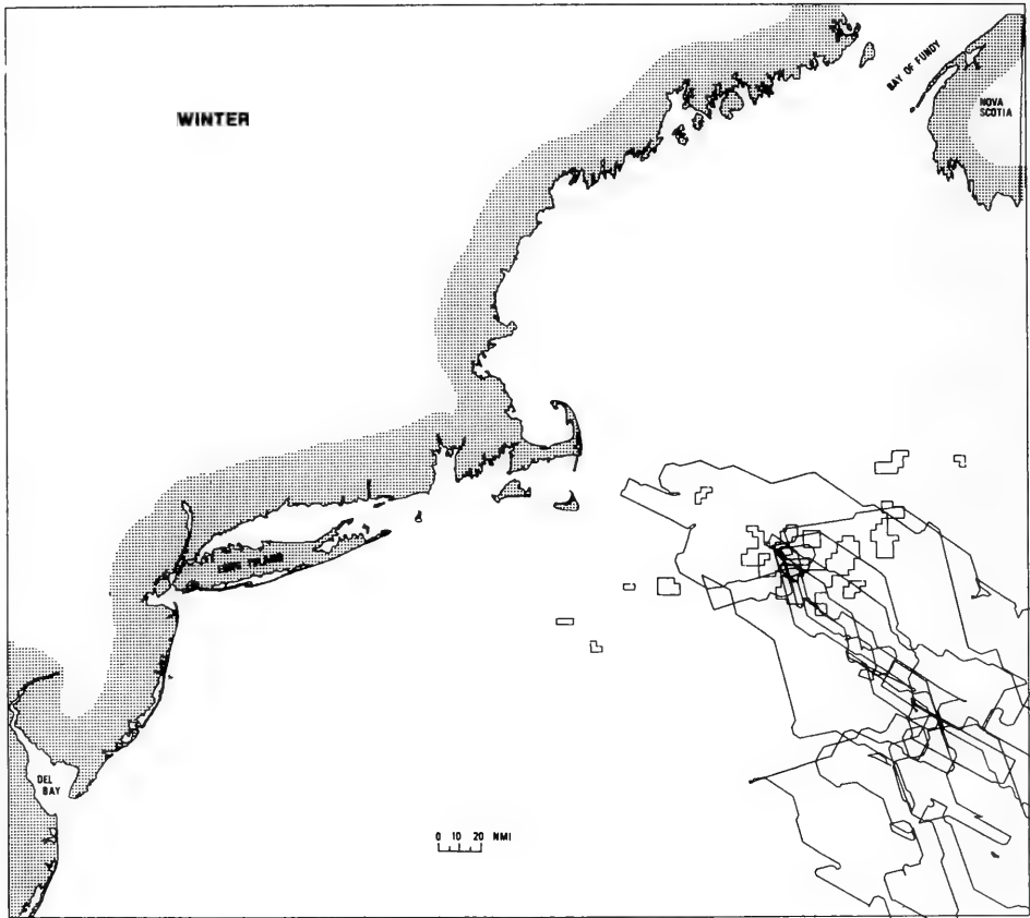
Figure 2-11. Example of oil spill trajectory results for the Georges Bank proposed lease area under winter conditions. (From Smith et al., 1976.)
