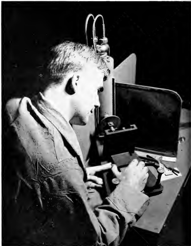
Multiple X-ray diffraction camera for studies in crystal structure and atomic distribution.
