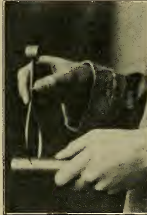
Fig. 17. Setting Calipers over a Mandrel.
