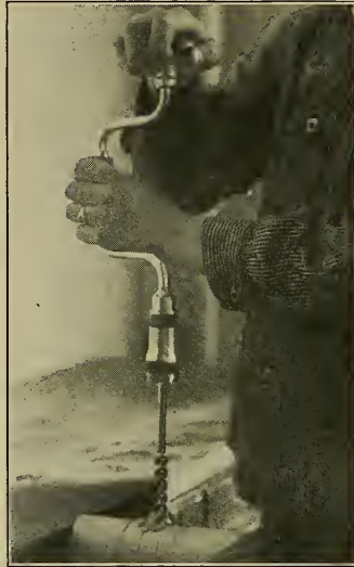
Fig. 34. Boring a Mallet Head.
