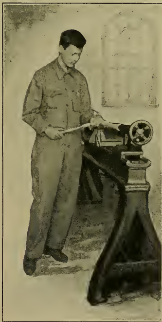
Fig. 12. Position at the Lathe.
