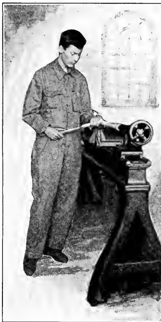
Fig. 12. Position at the Lathe.
