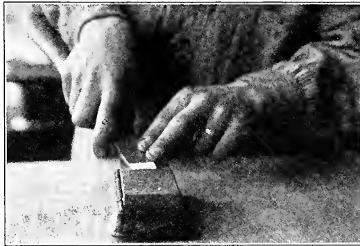
Fig. 8. Whetting a Skew Chisel.
