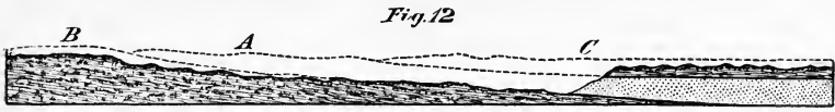
Figure 12 illustrates a common effect of erosion upon the surface area of the porous stratum, and the contour of the resulting basin. The dotted lines show the original contours.
